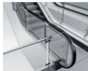
Passenger fall protection barrier height up to 1300 mm. Recommended when a fall greater than 6 m is possible
